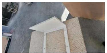
3) Align the other side piece to the right grove of the face panel and fasten with provided screws.
